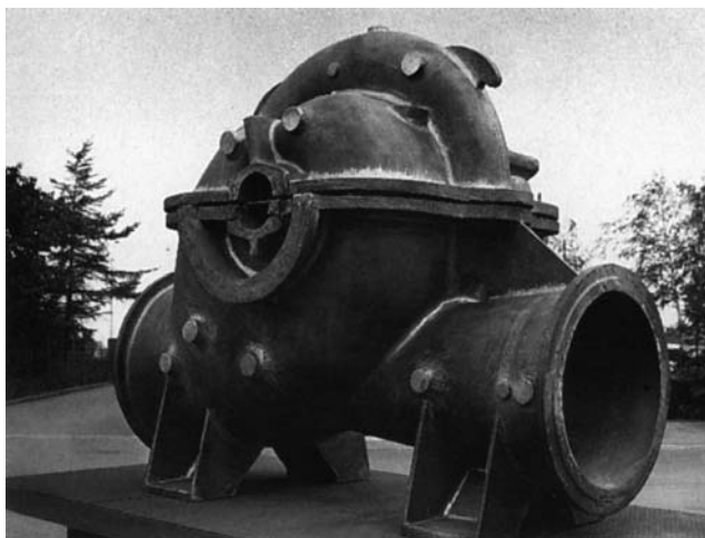
Two-part water pump for a desalination plant. Ni-Resist D-2W. (Klein, Schanzlin and Becker, Bremen, Germany)
