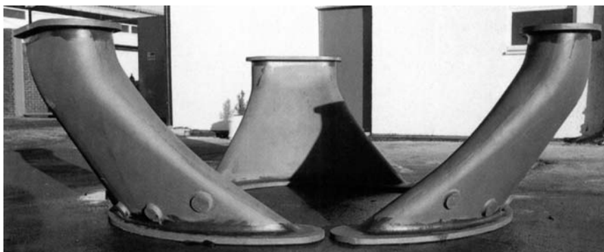
Hot air ducts for a variable temperature wind tunnel where operating temperatures can reach 580°C(1075°F). Ni-Resist D-2W. (The Taylor Group, Larbert, U. K.)
