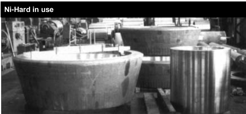
Loesche rolls for coal and cement grinding and roller for the clay and brick industry in Ni-Hard 4.
