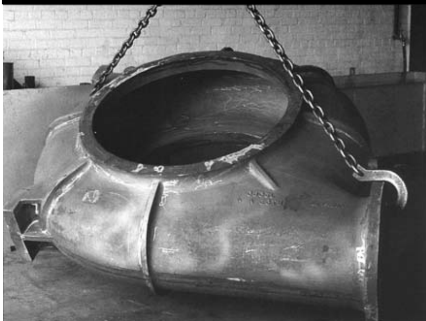
Casing in Ni-Hard 4 for sugar beet pump (900 kg)
