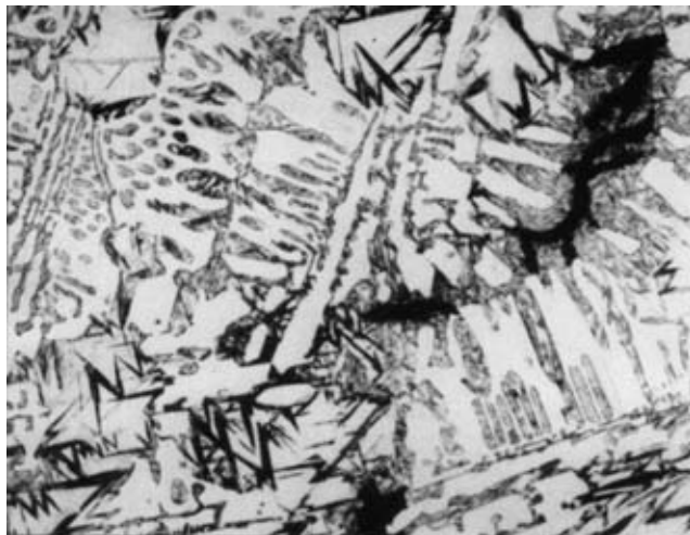
Figure 9. Graphite precipitates in the centre of a 50 mm plate section of Ni-Hard 1 with an unbalanced silicon content of 1.3%
