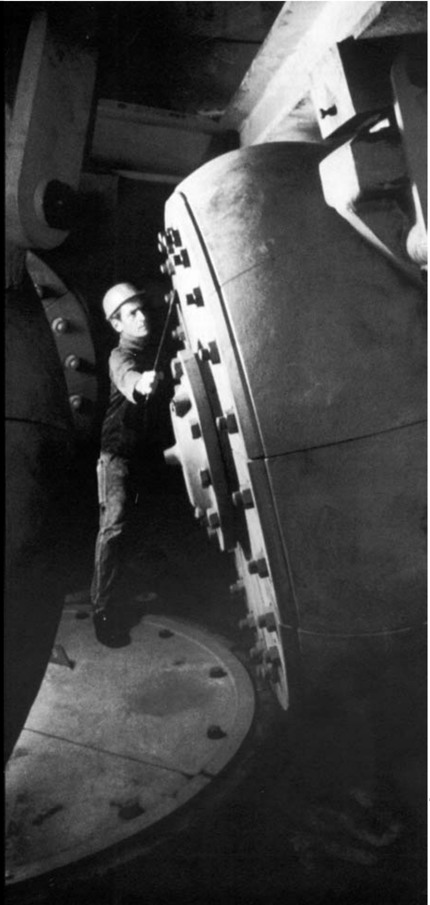
Pfeiffer roller pulverizer mill with segmented rollers and table in Ni-Hard 4 for limestone grinding, total weight around 80te
