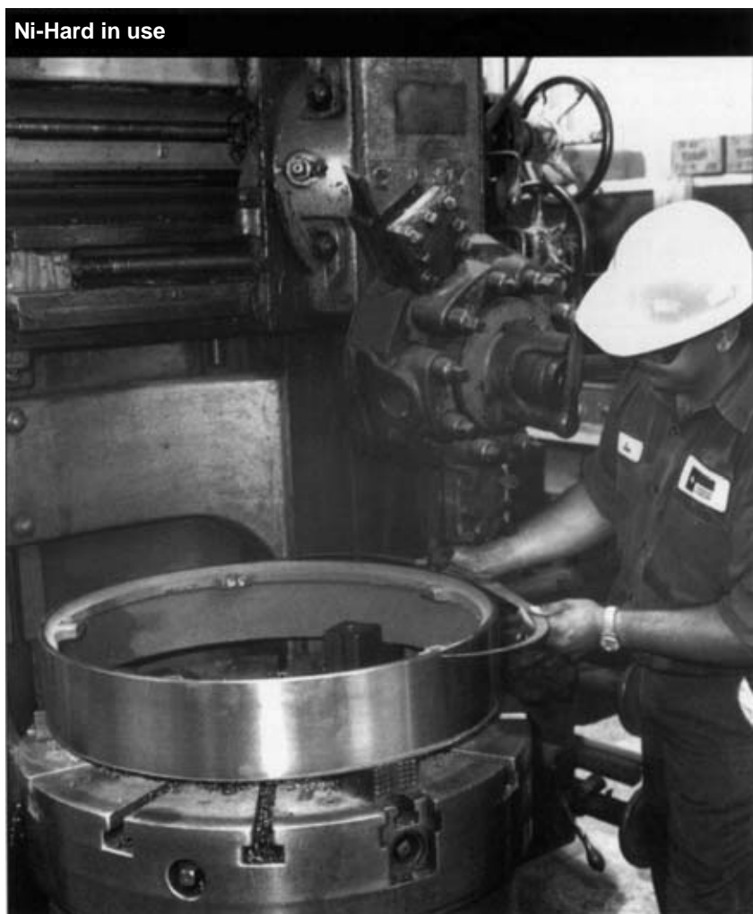
A 30-inch bottom or casing used in the production of concrete pipe. The Ni-Hard casing is machined using a CBN insert
