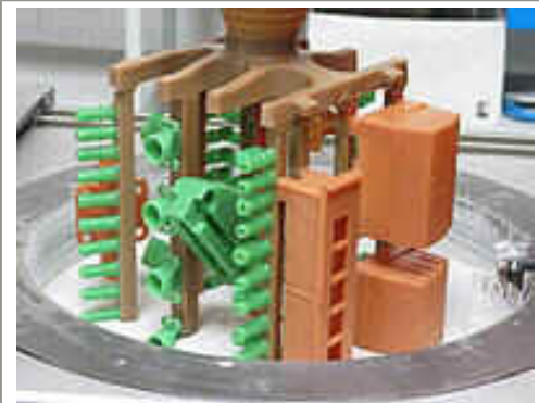
Wax Patterns Being Dipped in the Slurry (From MK-Technology.com)
