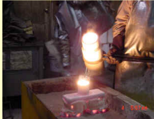
Metal Being Poured by Hand into the Mold
