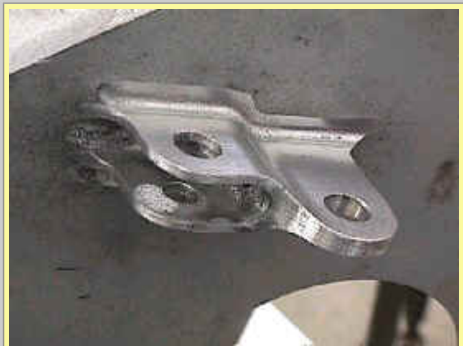
machined Clevis on Side Wall
