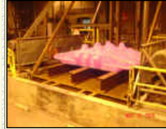
Hot Track Shoe Ready to Quench
