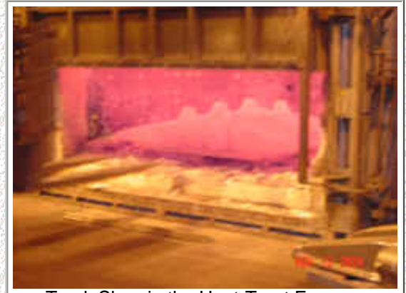
Track Shoe in the Heat-Treat Furnace
