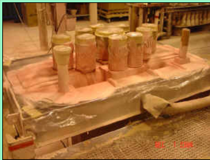
Pattern for Top Half (Cope) of the Mold
