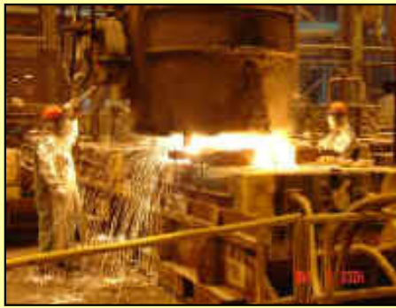
Metal Pouring into the Assembled Mold
