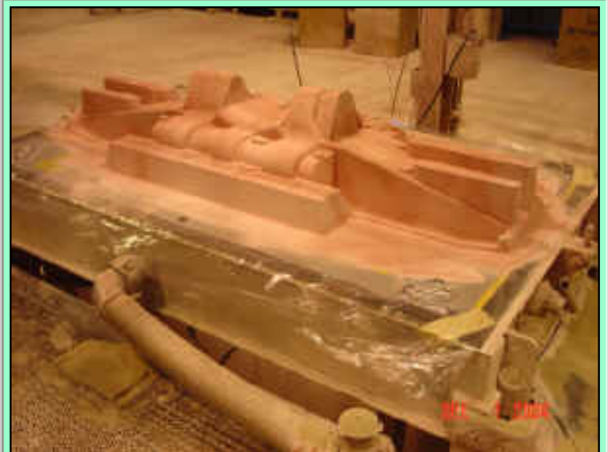
Pattern for Bottom Half (Drag) of the Mold
