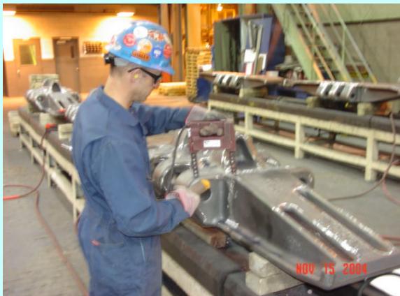
Magnetic Particle Inspection
