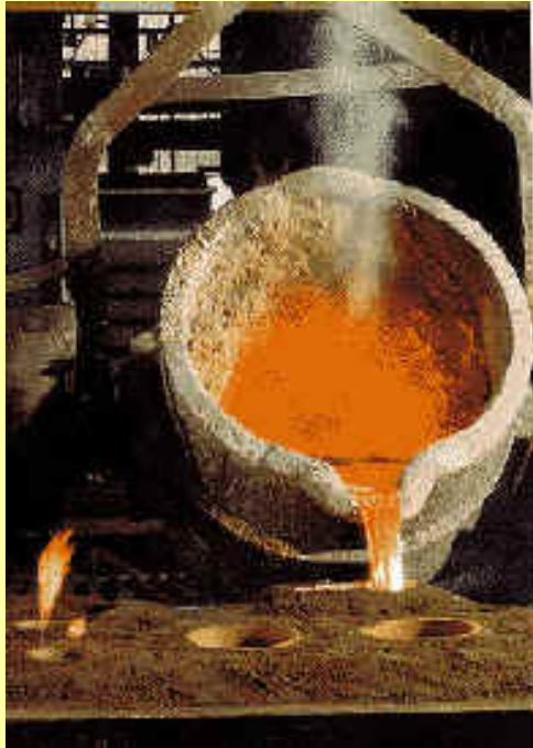
Metal Pouring into Sand Mold
