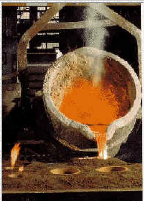
Metal Pouring into the Assembled Mold
