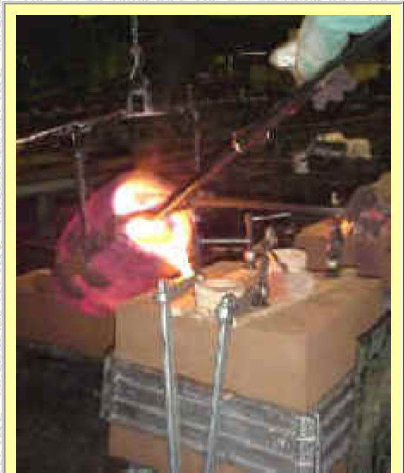
Metal Pouring into the Sand Mold
