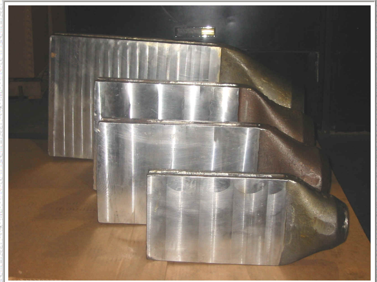
Cast Connectors Machined and Ready for Shipment
