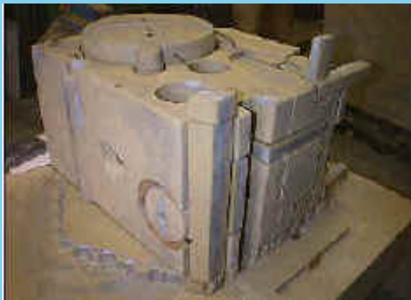
Interior Cores (Partial Assembly)
