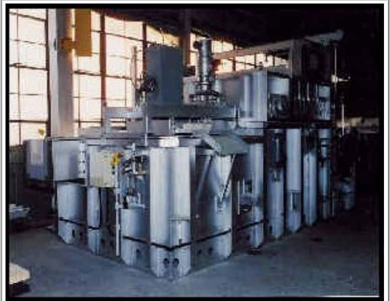
24,000 lb Electric Ladling furnace in Saginaw
