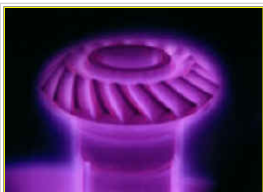
Component in Plasma Nitriding Chamber (from Rubig Plant Technology)
