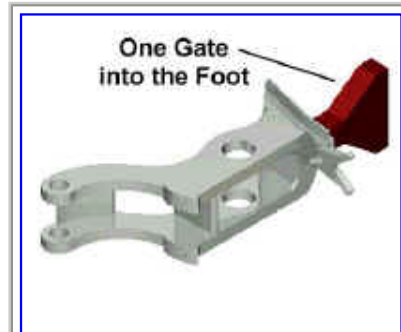
Option B -- One gate into the foot of the lever arm
