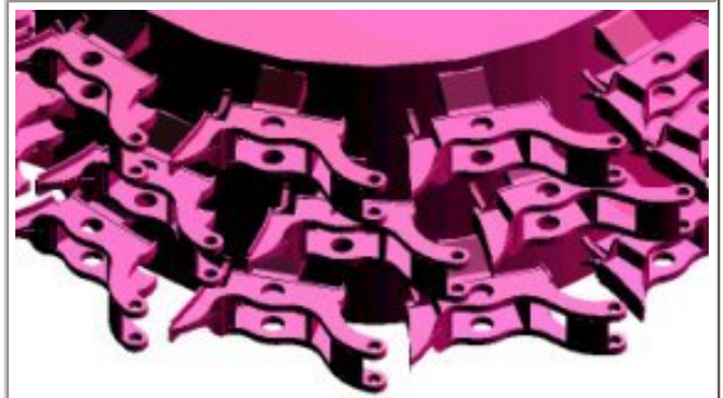
Option A -- Horizontal Orientation of Wax Patterns on Sprue
