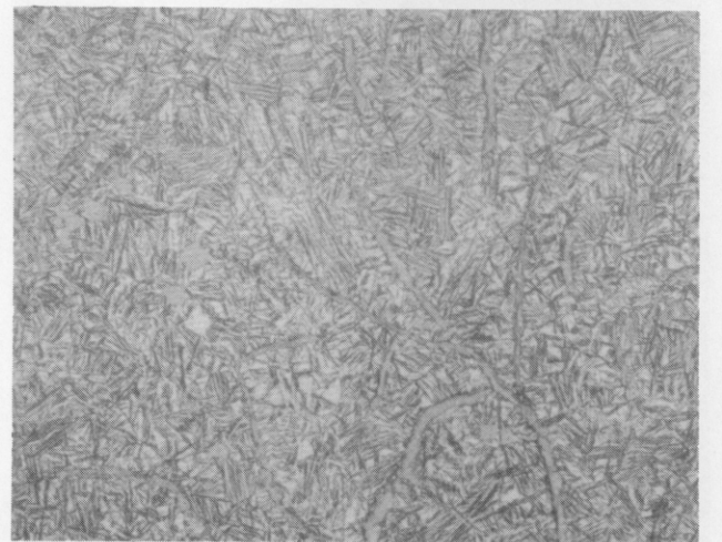
Fig. 9. Microstructure of Class 40 gray iron austempered at 700F (371C) for 60 minutes; 400X.
