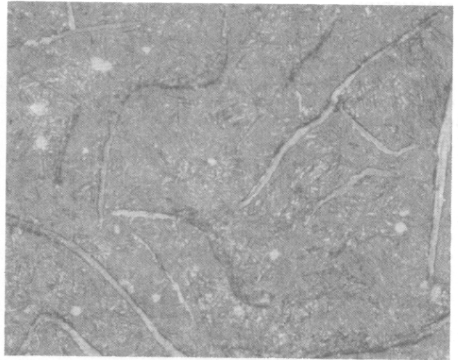
Fig. 13. Microstructure of Class 20 gray iron austempered at 500F (260C) for 180 minutes; 400X.
