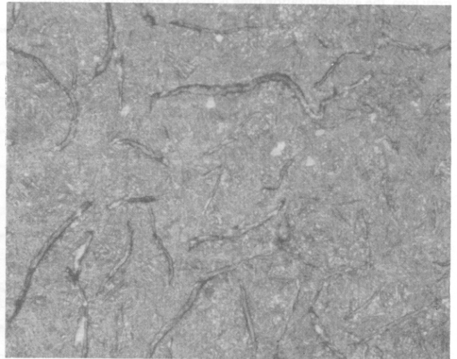
Fig. 14. Microstructure of Class 30 gray iron austempered at 500F (260C) for 180 minutes; 400X.
