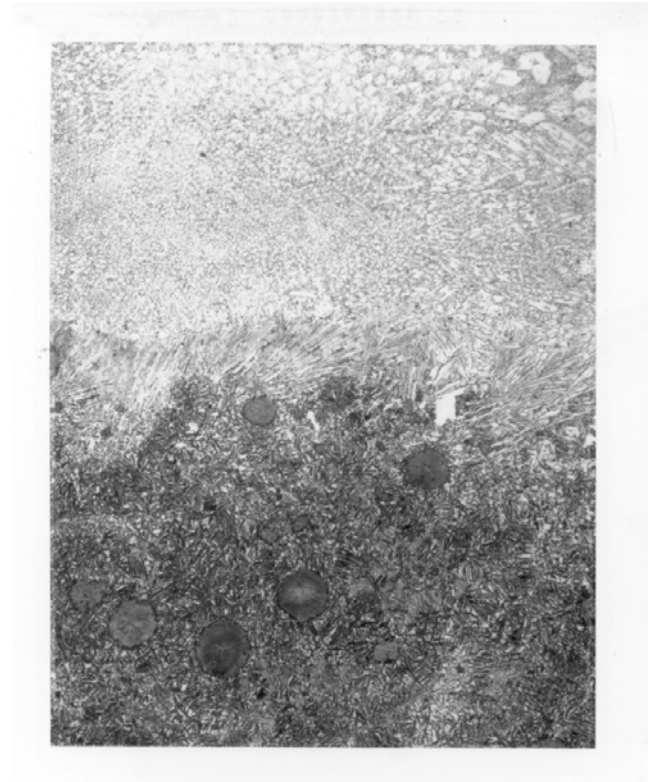
Figure 6: Microstructure of hard-face welded ductile iron showing the Carbide weld (light) and the pearlitic heat affected zone (dark).
