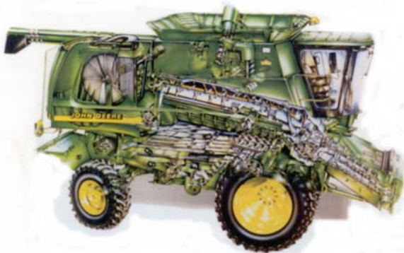
Figure 8: John Deere's new, high performance, rotary combine uses CADI in its critical threshing elements. (Courtesy of SAE Off Highway Magazine)
