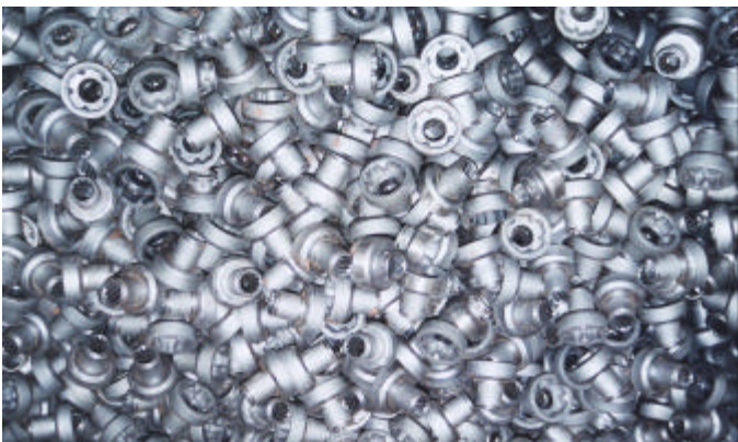
Figure 44: Carbo-Austempered™ Starter Clutch Shells
