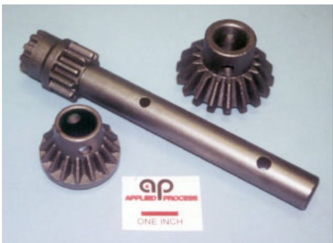
Figure 21 : ADI Trailer Jackstand Pinions with As-Cast Teeth
