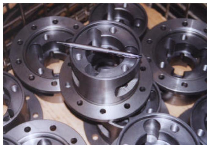
Figure 25 : ADI Limited Slip Differential Gear Housing
