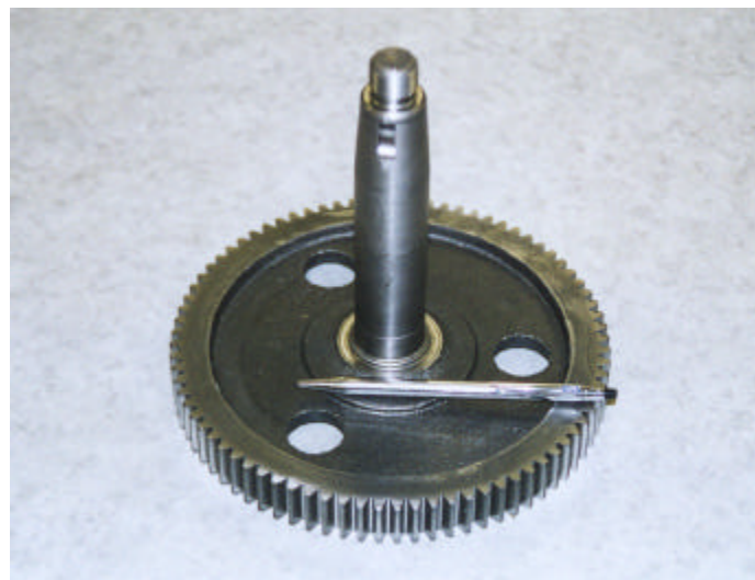
Figure 24 : ADI Gear and Axle for Commercial Lawnmowers.
