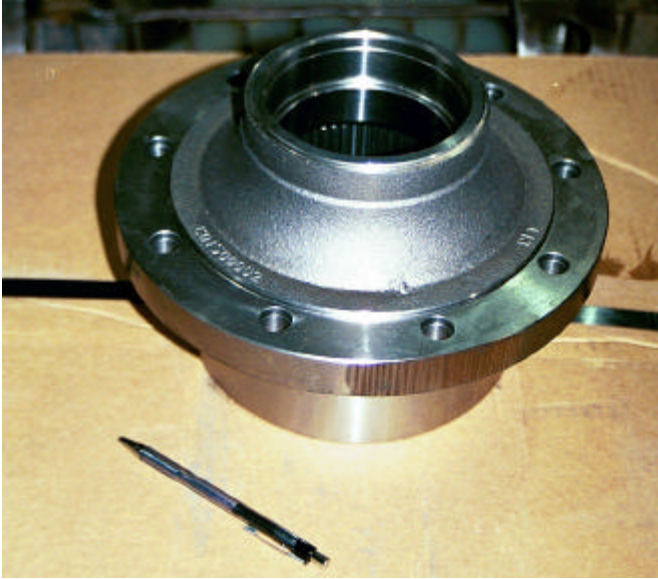
Figure 26 : ADI Grade 4 Scissor Lift Gear Housing
