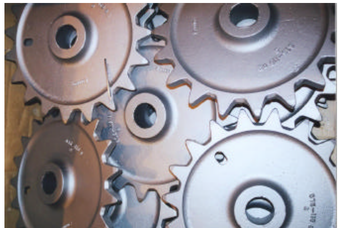
Figure 30 : ADI Sprockets for Crawler Type Construction and Agriculture Equipment
