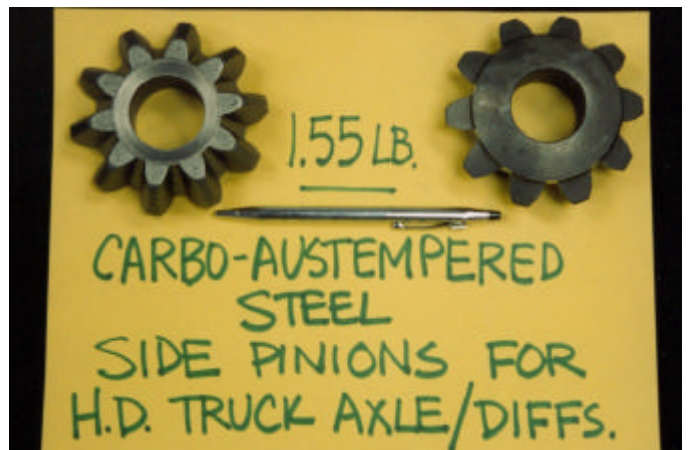
Figure 48 : Carbo-Austempered™ Steel Side Pinion
