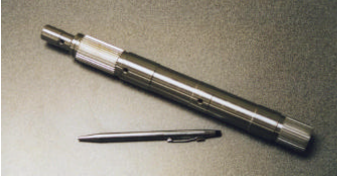
Figure 42 : Carbo-Austempered™ Steel Transmission Output Shaft for Medium Duty Truck and Bus (Courtesy of GM Allison Transmission)
