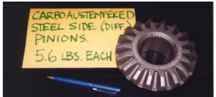
Figure 47 : Carbo-Austempered™ Steel Differential Pinion for High Performance Truck Axle
