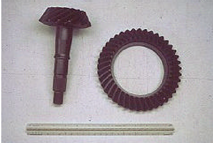
Figure 16 :GM ADI Hypoid Ring and Pinion Gears
