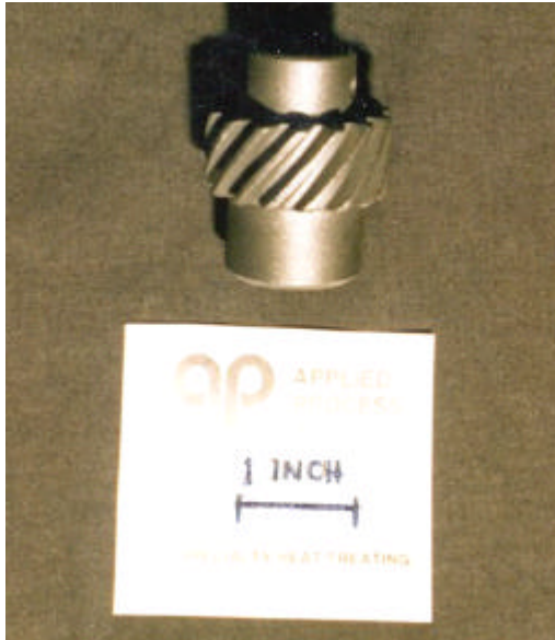
Figure 31: AGI Gear for Timing on a Light Vehicle Engine
