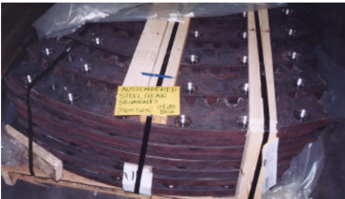
Figure 35: Austempered Steel Large Gear Segments
