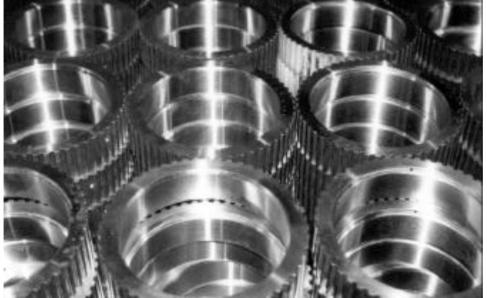
Figure 36 : Austempered Steel, Powdered Metal Sprag Races
