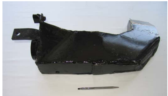
Figure 10: A rangeland seeder boot fabricated from cut, formed, punched and welded steel blanks.
