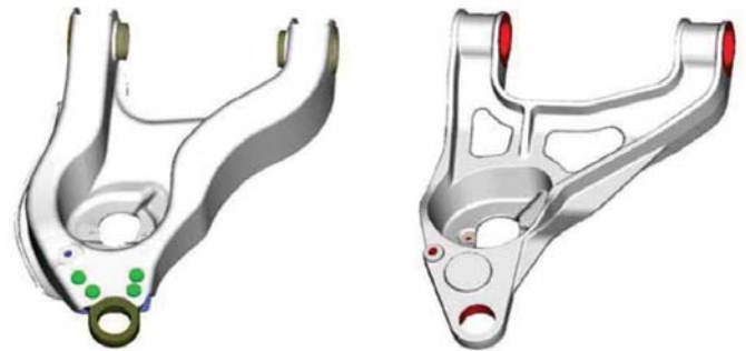
Figure 13: The ADI control arm (right) exceeded testing requirements and replaced the stamped steel component (left) at a 6% weight savings.
