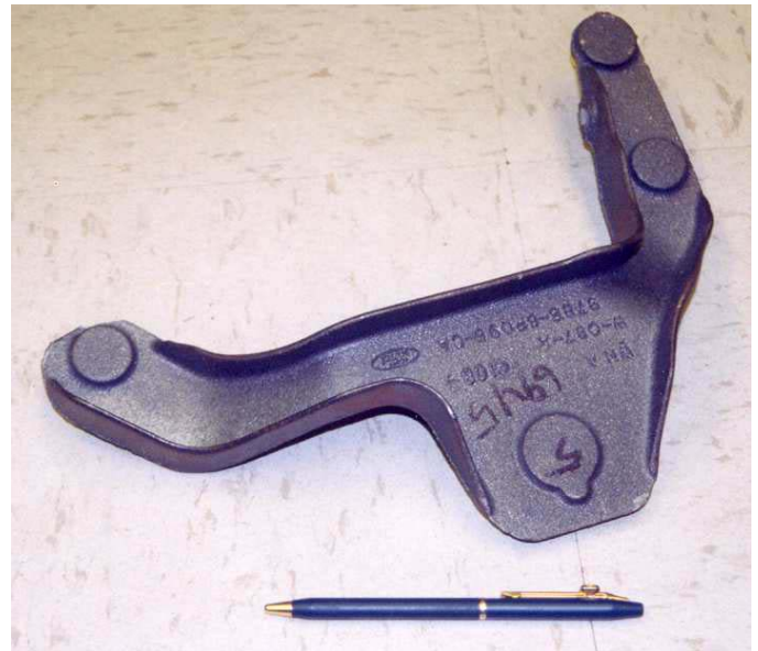
Figure 6: An ADI prototype bracket with a continuous 3mm wall.
