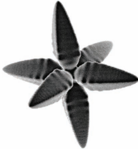
Figure 21. Phase field model prediction for a thermal dendrite with \langle 100 \rangle growth directions [36].
