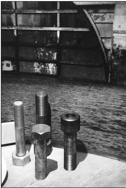
Typical stainless steel structural bolting. (Thames River Barrier)
