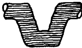
Bar Stock Grain flow broken by machining
