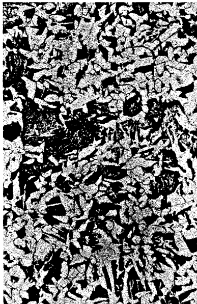
Fig. 36 A. Ferrite-pearlite structure—representation in a 1.5-in. (38 mm) section of a larger 15-ton, 2% Ni, .20% C steel turbine blade casting that was normalized and tempered. B. Same as in A, but coarser and acicular Widmanstätten structure in the center of a 7-in. (178 mm) thick portion of the same casting. C. Same as in B, but coarse and blocky in appearance in the center of a 28-in. (711 mm) thick portion of the same casting.
