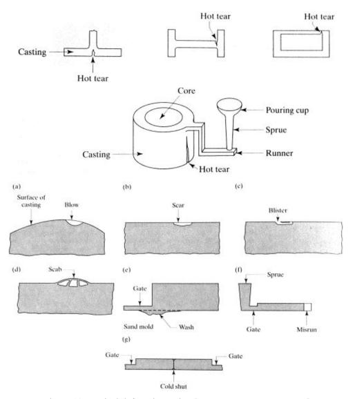
Figure 13. Typical defects in casting [source: Kalpakjian & Schmid]
