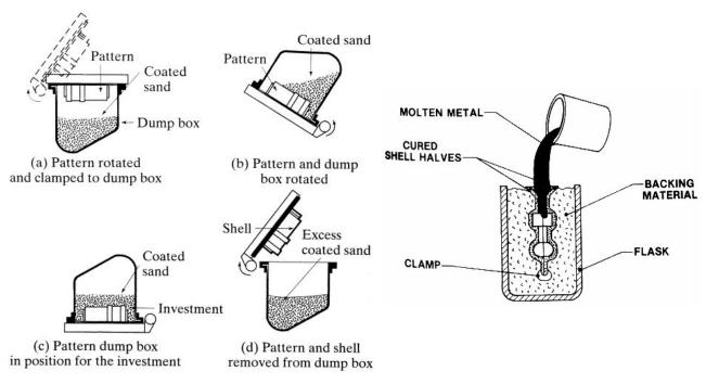
Figure 5. Making the shell-mold [Source: Kalpakjian & Schmid] Figure 6. Shell mold casting
