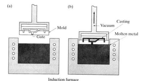
Figure 9. Vacuum casting [source: Kalpakjian & Schmid]
