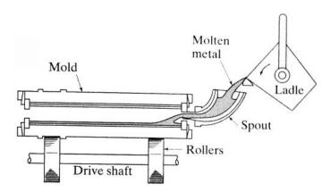
Figure 12. Centrifugal casting schematic [source: Kalpakjian & Schmid]
