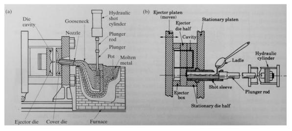
Figure 11 (a) Hot chamber die casting (b) Cold chamber die casting [source: Kalpakjian & Schmid]
