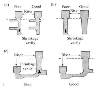
Figure 18. Poor and preferred design examples [source: Kalpakjian & Schmid]
