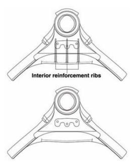
Figure 17. Adding ribs to flat region decreases warping and increases stiffness against bending moments
