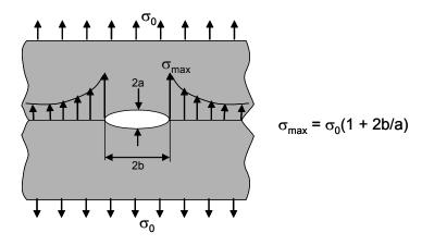
Figure 14. Stress concentration near an elliptical defect
