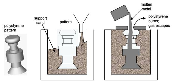
Figure 7. Expendable mold casting
