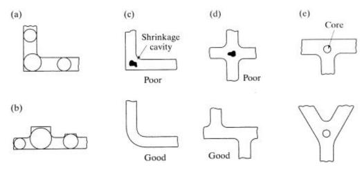
Figure 16. Poor and preferred design examples [source: Kalpakjian & Schmid]
