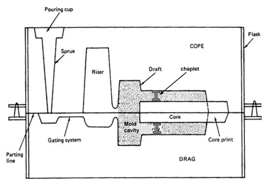
Figure 4. Design components of a mold showing chaplets
